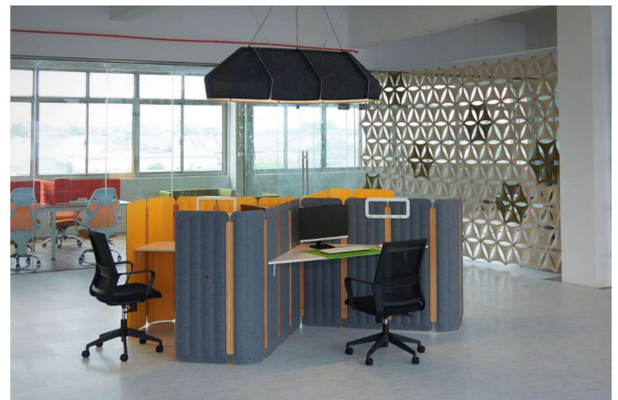
Use acoustic partitions to help manage noise in both quiet and loud zones.
