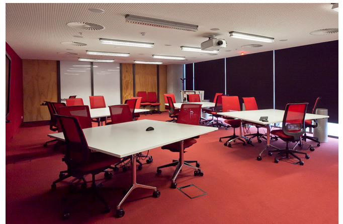
Conference rooms can be very noisy, additional acoustic panels along the walls and the ceiling, as well as carpet can do a lot to absorb noise and prevent noise propagation into quiet work zones.
